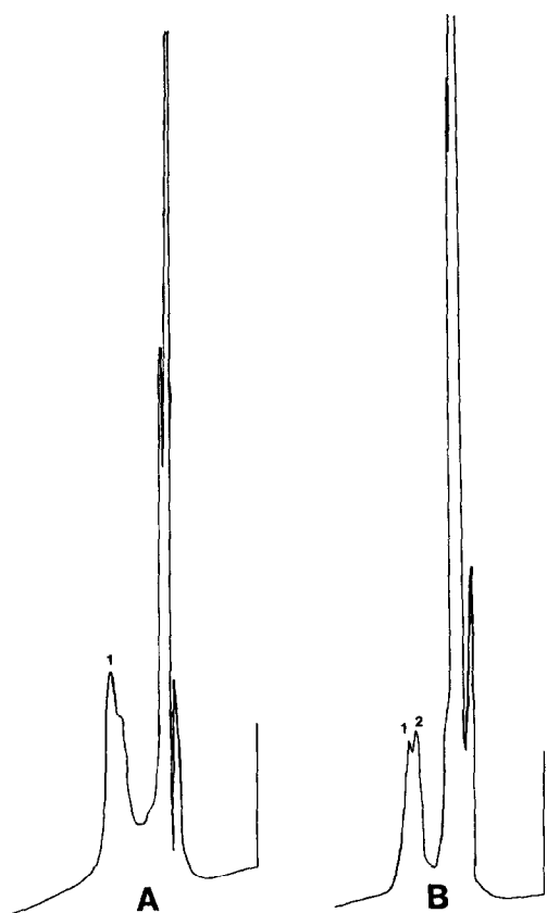
Fig. 3. Reversed-phase chromatographic behaviour of \beta -endorphin as a result of changes in sample solvent composition prior to injection onto the HPLC column. Chromatograms are those which were gained when a sample of \beta -endorphin was reconstituted with either (A) \text{CH}_3\text{CN-KH}_2\text{PO}_4 , pH 2.3 (40:60) or (B) \text{CH}_3\text{CN-KH}_2\text{PO}_4 , pH 2.3 (50:50). The first and second eluting peaks are denoted by 1 and 2, respectively. Isocratic mobile phase constituents were \text{CH}_3\text{CN-KH}_2\text{PO}_4 (adjusted to pH 2.3 with Aristar \text{H}_3\text{PO}_4 ) (32:68).
